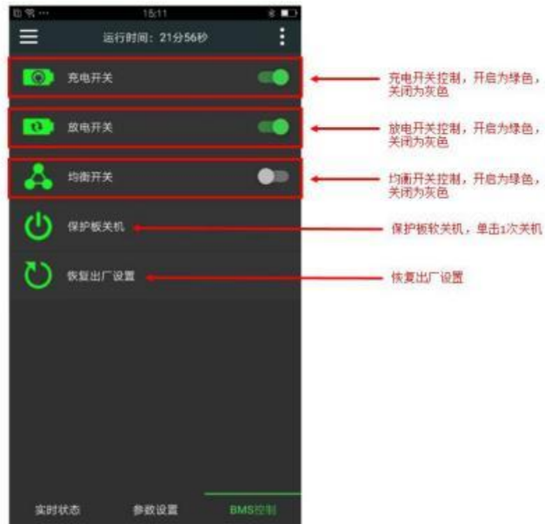
picture 15 BMS control page
