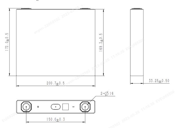
Fig.7 Diagram of Cell Size and Appearance 图 7 电池尺寸及外观图
