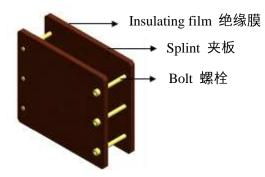
Fig. 2 Diagram of the clamp covered with insulation film 图 2 电池夹具包绝缘膜图
